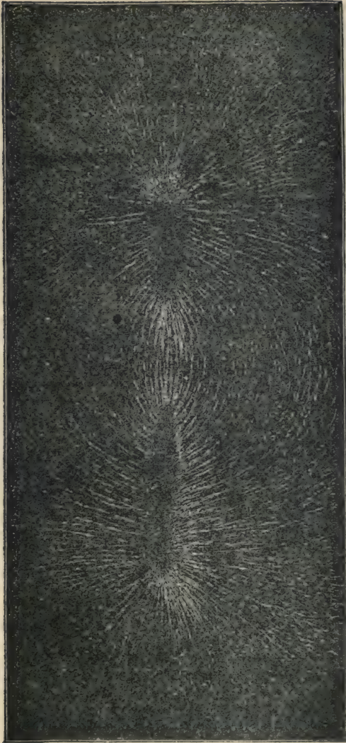
MAGNETIC LINES OF FORCE. From a Photograph by PROFESSOR MAYER.
